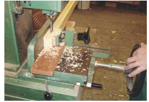
▲ Pic.12 ...ready for mortising, a task that Mike carried out on, well...the mortising machine!
